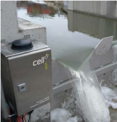
Flow measuring point in a watercourse with a triangular and rectangular notch weir combination. Battery operation for flow and temperature measurement.
