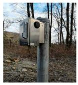
Compact design installed on the water level tube of the groundwater measuring point with alternating battery operation
