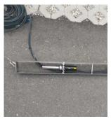
Stable and expandable probe suspension device for hanging in groundwater measuring points or wells
